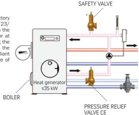
Thanks to the highly precise setting (up to  $\pm 0.1$  bar), to the variety of available seat gaskets(brass, rubber and PTFE) and to the different types (free or conveyed discharge), they can be used in several systems, also systems on compressed air and steam. Free and Conveyed discharge-type safety valves are factory set and sealed; responding to the requirements laid out in EU Directive 97/23/EC (PED) for pressure equipment, and are therefore classified as Category IV and bear CE 1115.
